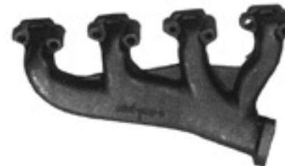
HERE IS AN IMAGE OF AN EXHAUST MANIFOLD AS FOUND IN A CAR.
